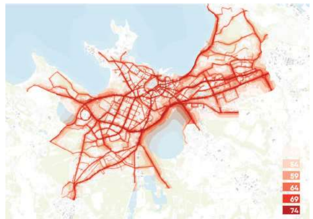
Figure 3.26. Road traffic noise map of the streets of Tallinn. Source: Daily Road Traffic Noise Map of Tallinn, 2015.
