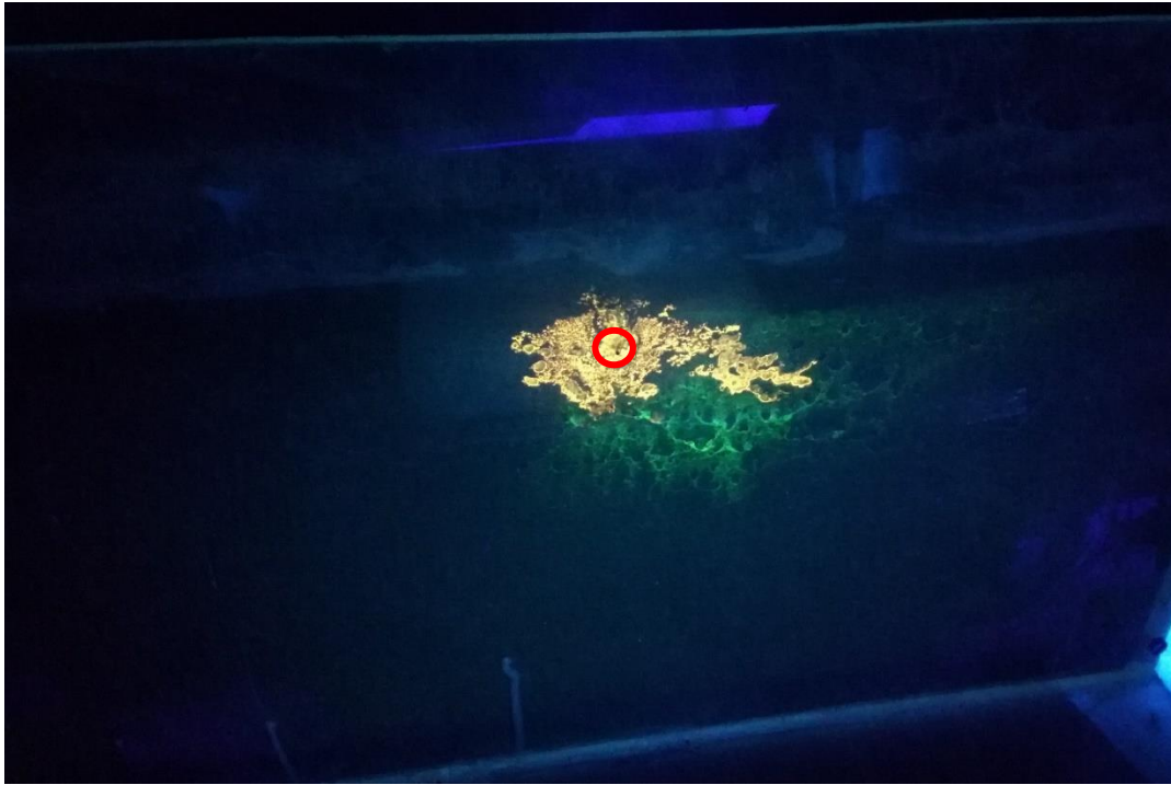
Figure 2.3. Situation before switching on the electric current - the greenish water-soluble color had started to spread, whereas the oil color had mainly remained in place. The injection spot is marked with the red circle.
