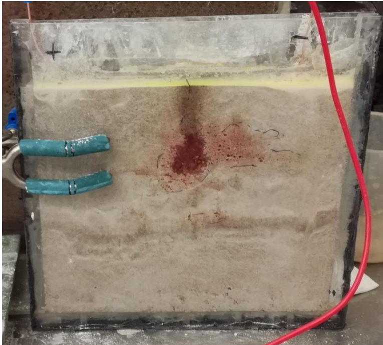
Figure 2.8. The situation immediately after switching on the electricity. The water-soluble fluorescein (yellow color) had migrated towards the surface. The spreading before electricity has been marked with a black dashed line.
