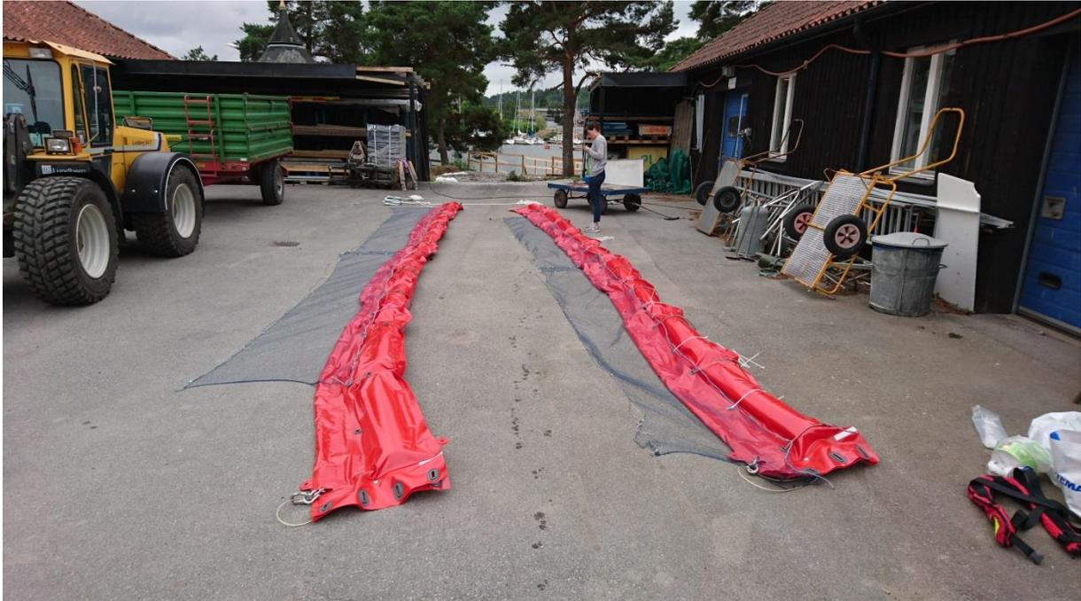
**Figure 1. Litter booms (C500) equipped with net curtains.**
