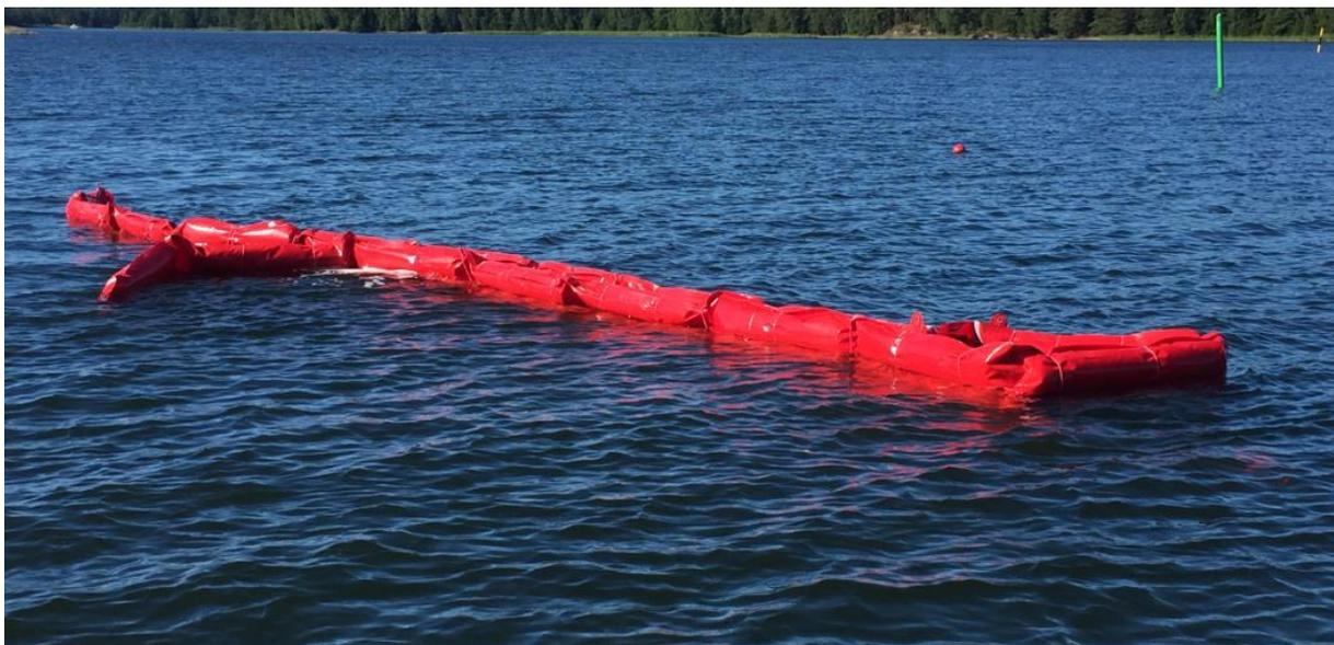
**Figure 16. One mooring point of Boom 1 came out of position resulting in a deformation of the litter boom. It was not able to capture any litter.**
