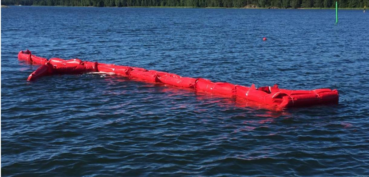
*Figure 3. Strong winds resulted in a deformation of the litter boom. It was not able to capture any litter.*
