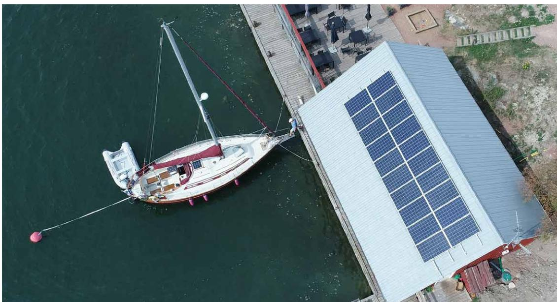
Figure 19. An on-grid PV system was installed on the rooftop of a restaurant building in Sottunga port. © Kristiina Kortelainen
